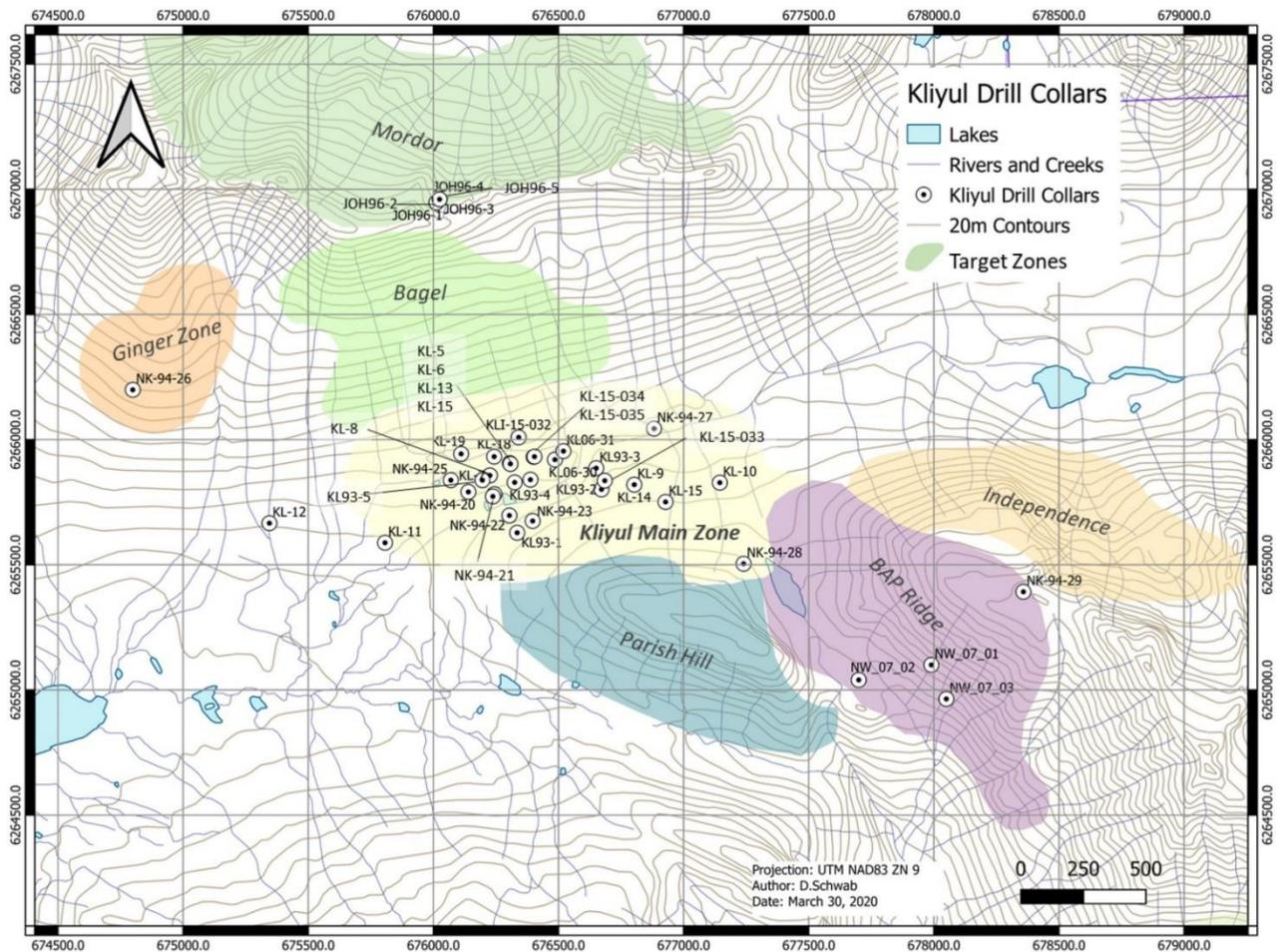
Figure 6.3 Kliyul drill hole plan map. Source: Pacific Ridge (2020).
