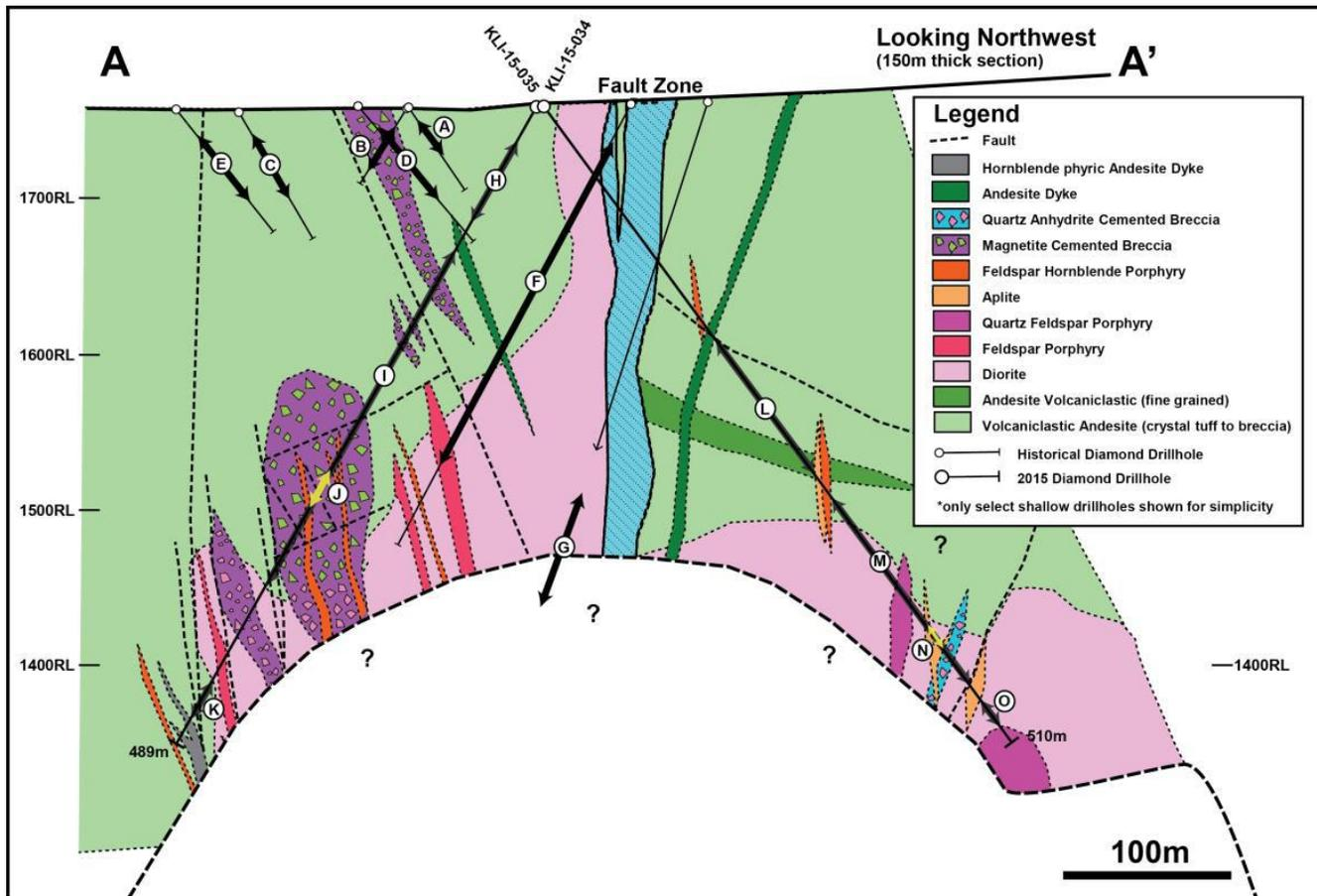
Figure 6.5: Kliyul Main Zone drill cross-section. Refer to Figure 6.4 for cross-section location and Table 6.4 for drill intercepts denoted by capital letters. Source: Pacific Ridge (2020)
