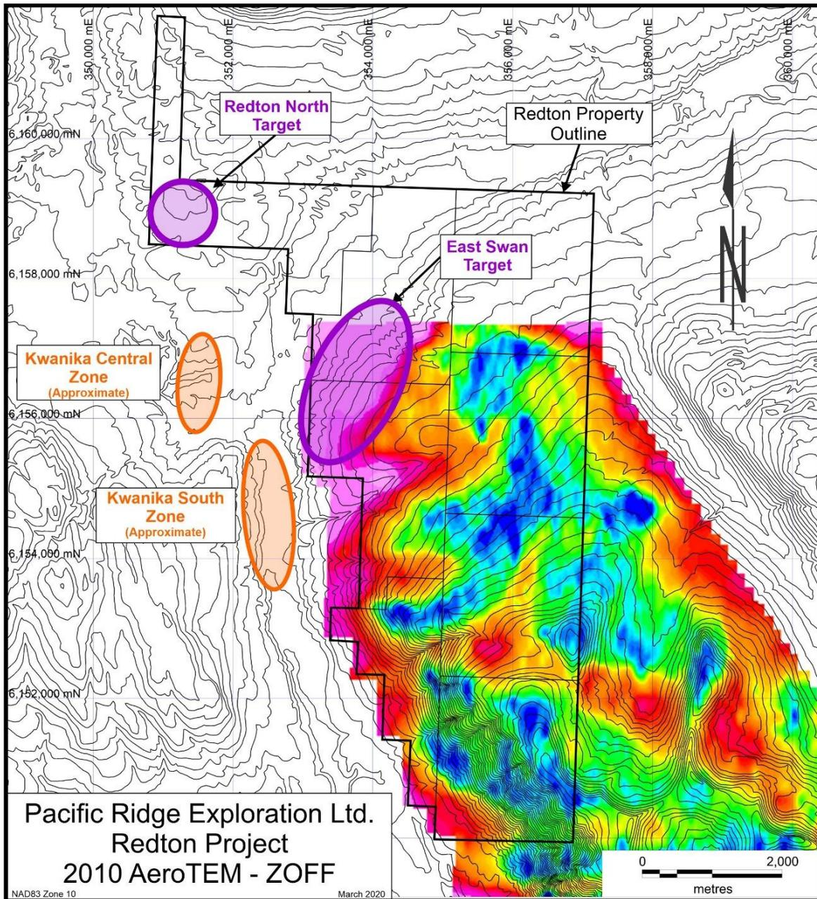
Figure 6.6. Swan East Target – AeroTEM conductivity (Zoff). Source: Pacific Ridge (2020)
