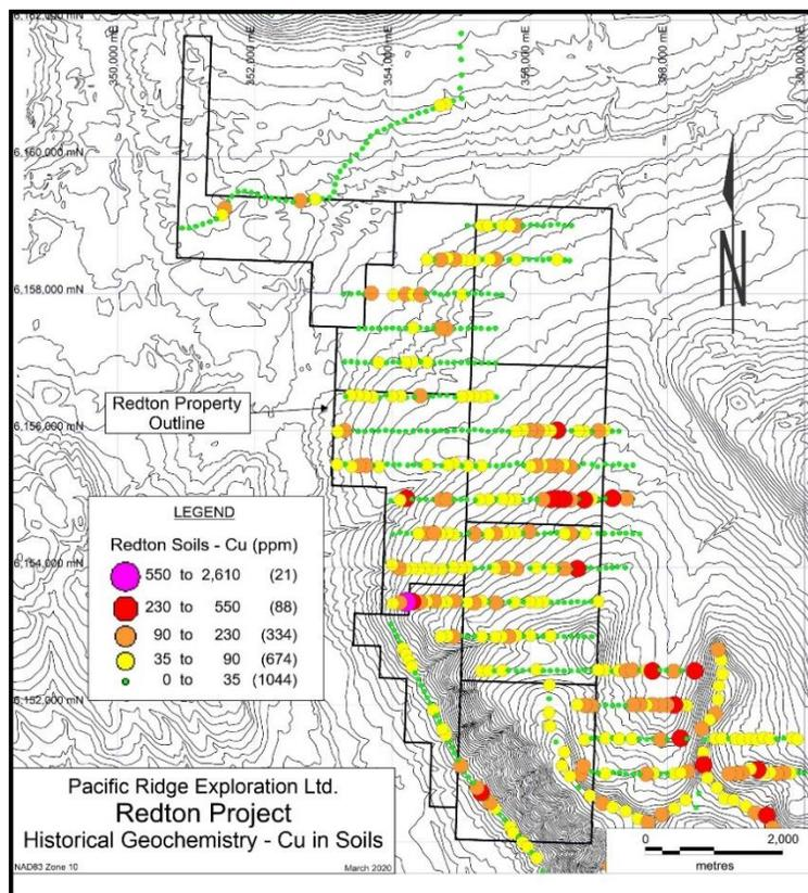
Figure 6.7. Soil geochemistry – copper. Source: Pacific Ridge (2020).
