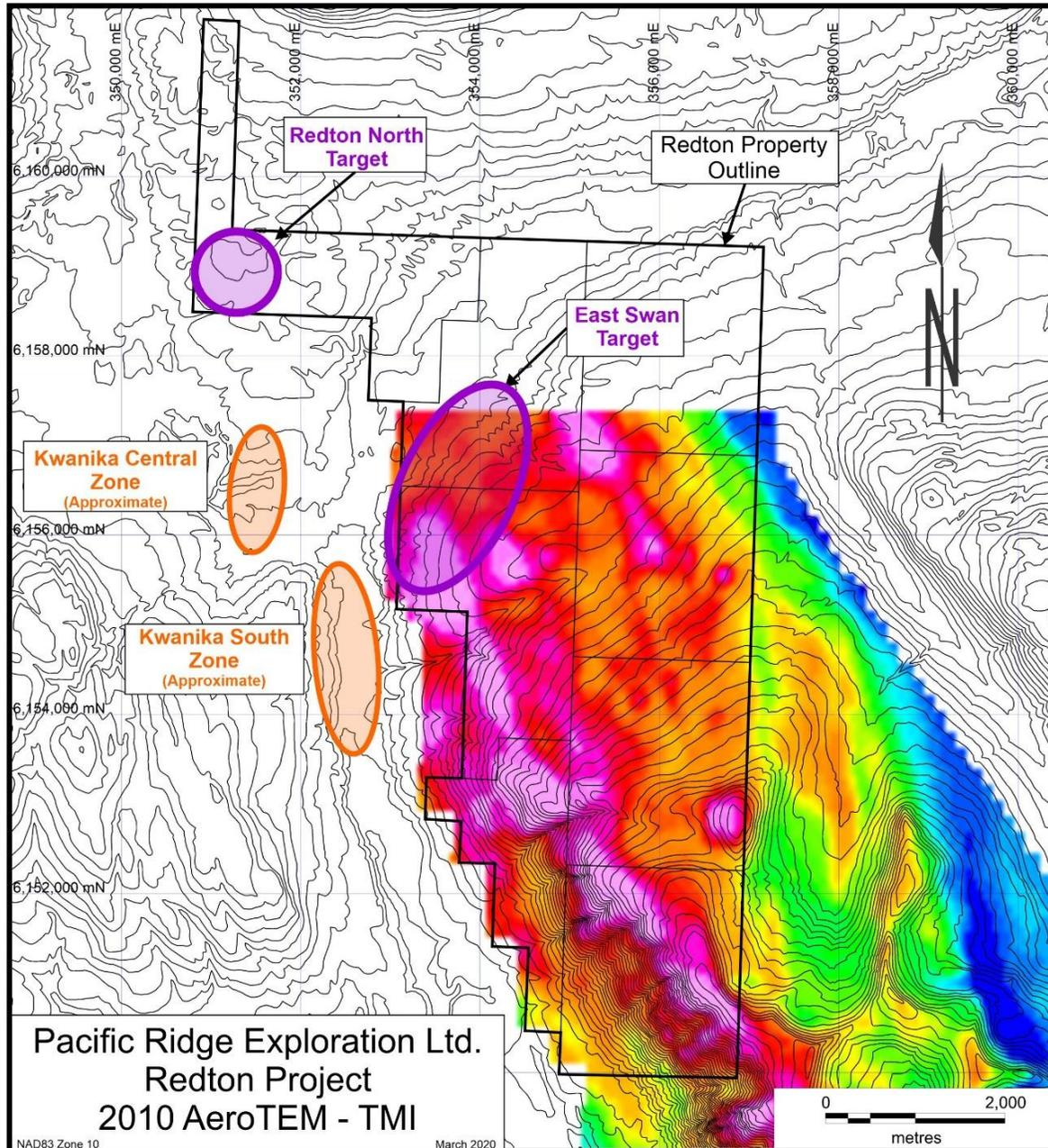
Figure 6.5. Swan East Target – AeroTEM total magnetic intensity. Source: Pacific Ridge (2020)
