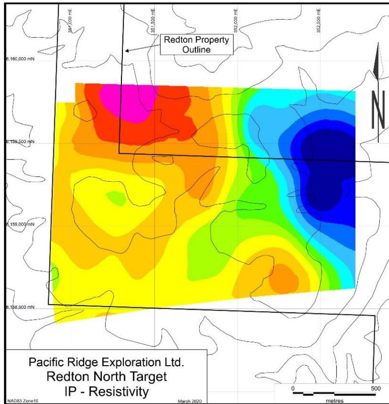
Figure 6.3. Redton North target – IP resistivity. Source: Pacific Ridge (2020).
