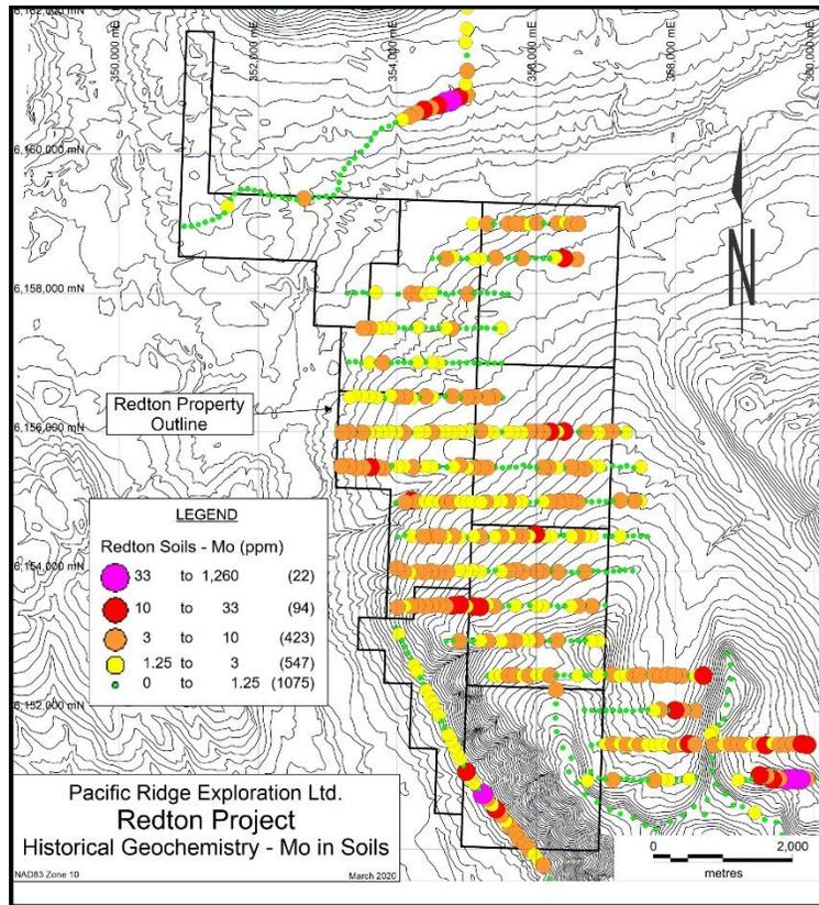
Figure 6.8. Soil geochemistry – molybdenum. Source: Pacific Ridge (2020).
