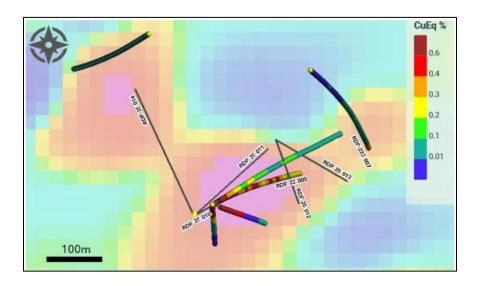
RDP-25-010, the first drill hole of the 2025 exploration program, was located 40 m southwest of RDP-22-005. RDP-25-010 was drilled at an azimuth of 60° degrees and dip of 72°. A stockwork of quartz-magnetite-sulphide veins was encountered in the first 5m of drilling, however, a late mineral intrusive was intersected from 5m to 175.5m and the hole was terminated.
